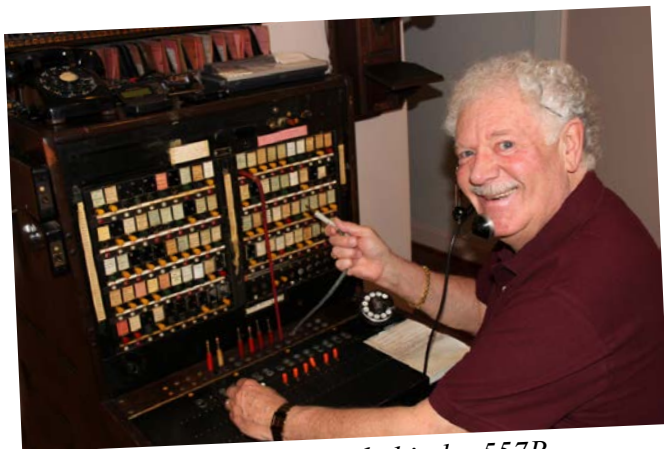
Here Steve Michaels slips behind a 557B cardboard. The difference between the 557A and 557B is that the phone dialing pad is at the top versus the bottom
